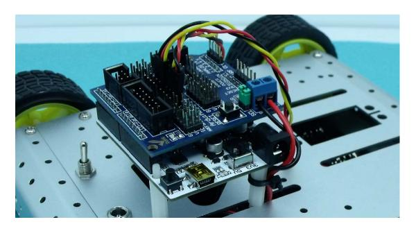
Extender board connected to the control, it can be change according to the program.
