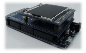
LCD-2000-NT3916/ILI9225/ST7775  $\times$  UNO R3  $\times$  Adapter plate
