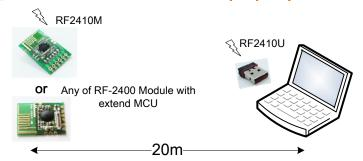
RF-2410U used as a RF receiver, can be connection to any of RF-24xx series module, note the RF2410M is MCU based and it can be work alone as a independent device.
