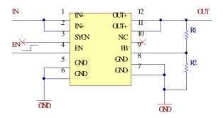
The picture shows a typical application of the PM-XXXX series. It is not every module has SYNC pin and FB pin, they should be connected depending on the application. The other pins are connected in the same way.
