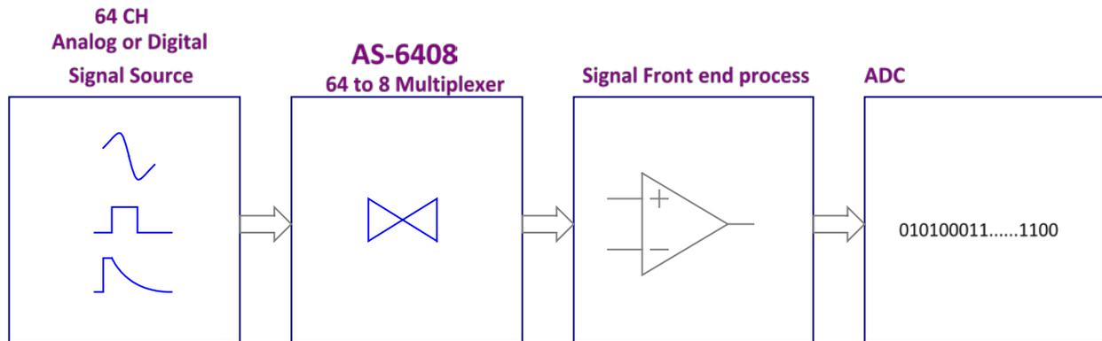
AS-6408 have two output ways, one is 64CH  $\leftrightarrow$  8CH and one is 64  $\leftrightarrow$  1CH, the 1CH output is after the 8CH output and they can working at the same time.
