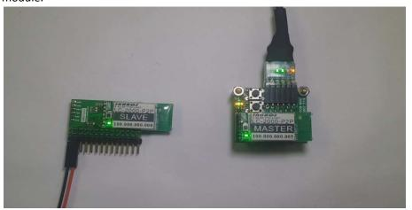
2. Then we press the pairing button on the Master-side, it turn to the pairing state, press again, the module turn out of the pairing state. Similarly, we have to look at the changes in Slave-side.
