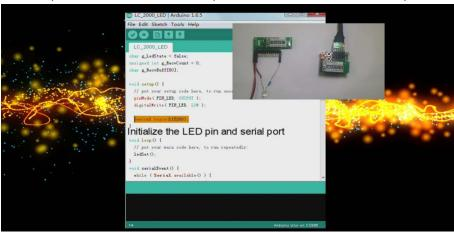
In the loop function, we just need to call the LED control function.
