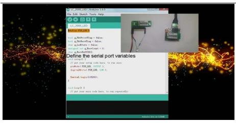
The set up function, initialize the LED pin's state and initialize the serial port baud rate, set the baud rate to 115200bps.
