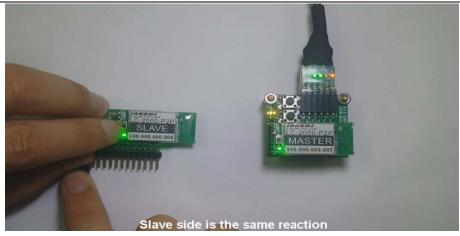
3. Pairing is completed, the lamp of the two sides are light off.
