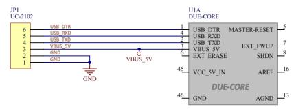
**Power Connection 2:** powered by VCC\_IN\_5V, in this case , The VCC\_5V\_IN must limit tolerance within +/-5% , which means the voltage range is 4.75-5.25V. The connection as below :
