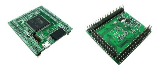
DUE-CORE is a compact version of DUE, It integrates all peripherals required for MCU, and all GPIO are connected to the 2.54mm connectors for users. As a standard MCU core board, apart from main features with DUE also has the following features:
