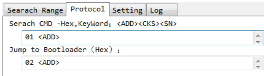
**<ADD>** : it’s the hardware address which set by 5bit coder, range 0 to 31, Hex range is 0x00 to 0x1F.
