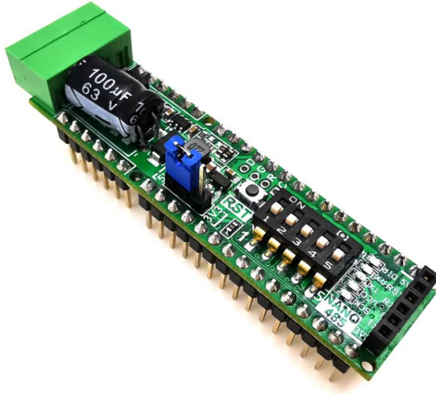
NANO485 inherits the pin assignment of the standard Massduino NANO and expands more IO pins, so the NANO485 is slightly longer than the standard Massduino NANO.
