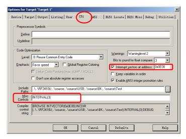
Checked "Interrupt Vector At Address" box, and set to "0x0E00";
