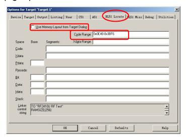
Uncheck "Use Memory Layout from Target Dialog" box, fill "Code Range" with "0x0E40-0X3BF6" o
